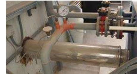
Gas Filtering and Sampling System
